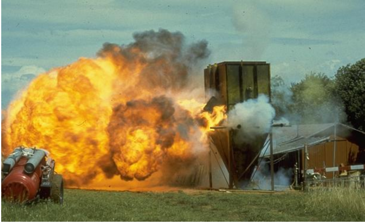
Figure 8-4. Dust explosion in a filter housing with additional deposits of loose dust near the venting area by standard dust dispersion
