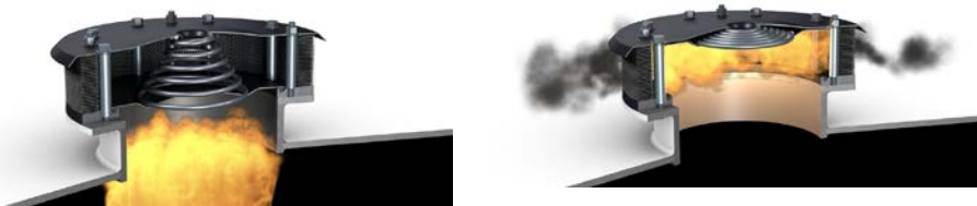
Figure 10-7. Schematic representation of an explosion relief valve system; left: closed; right: open during explosion /26/
