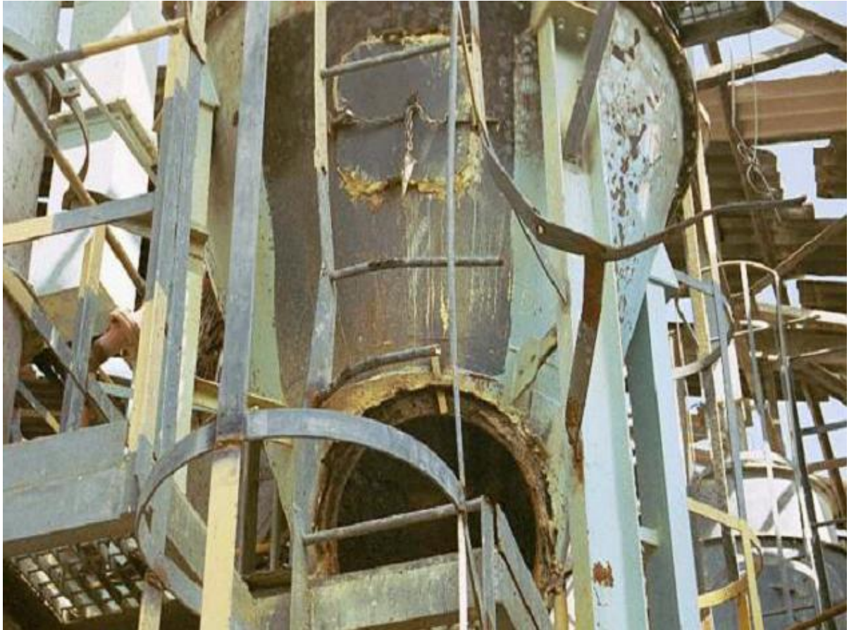
Figure 6-1. Consequences of poor vent design
