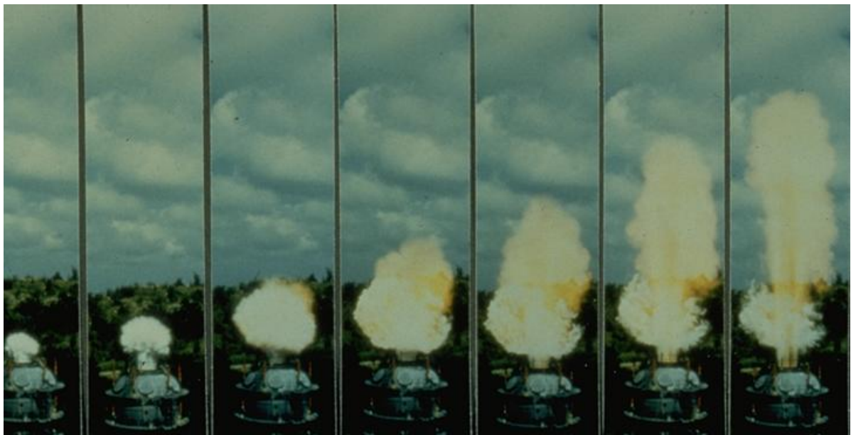
Figure 8-3. Dust explosion in a 250-m 3 -vessel with standard dust dispersion, venting upwards
