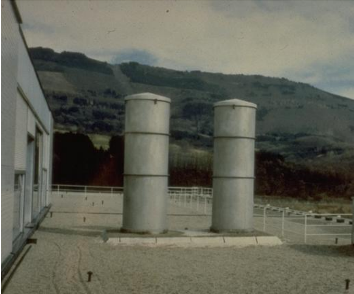
Figure 9-15. Tested metal covers held by rubber bands (the retaining wires for the covers are not visible)
