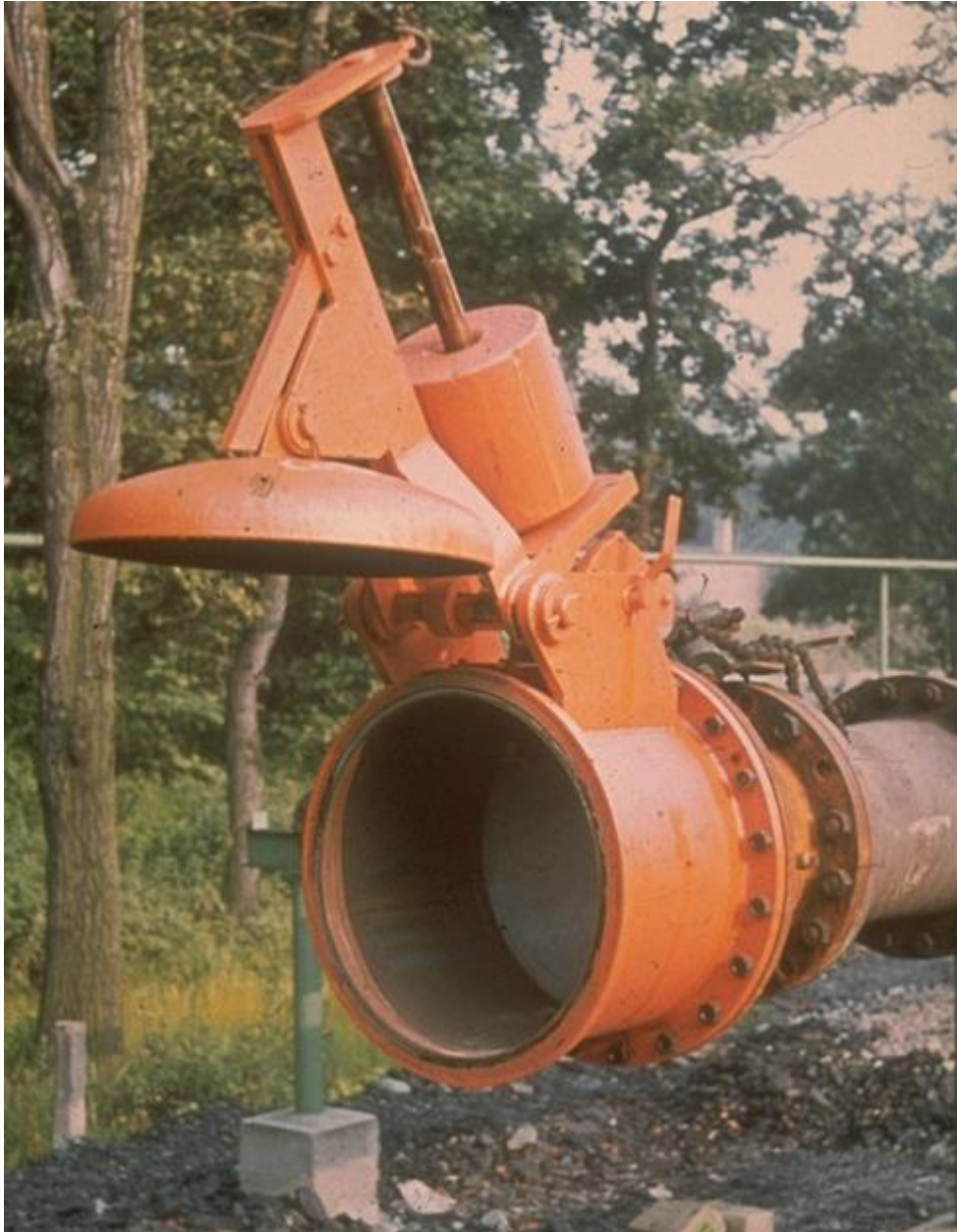
Figure 13-3. Venting device at end: Counter-balanced, hinged explosion door /5/
