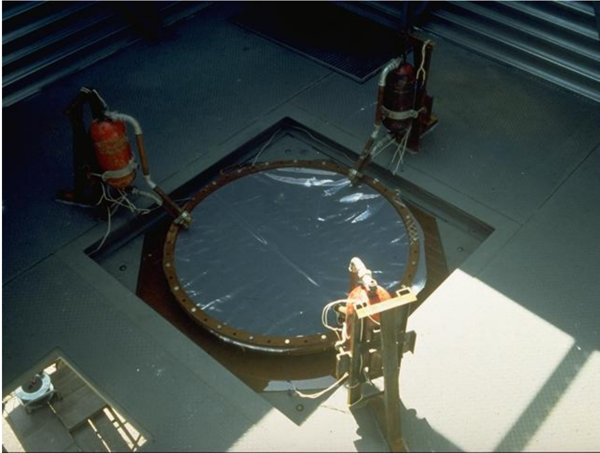
Figure 6-20. Extinguishing barrier inside the silo floor close to the vented silo top
