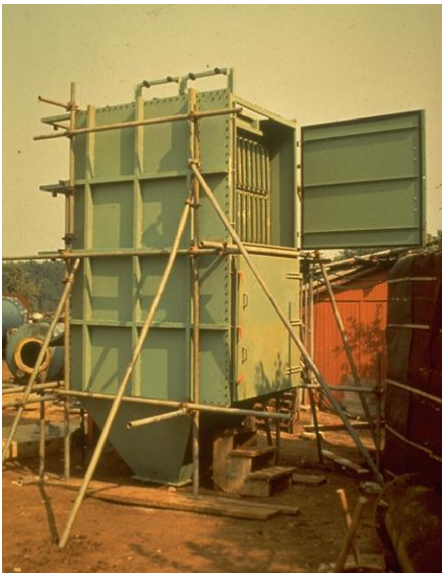
Figure 6-11. Pocket filter with filter elements: Filter volume (dirty volume) = 7.5-m 3 ; Volume of the filter elements = 2.5-m 3 ; Free dirty volume = 5-m 3
