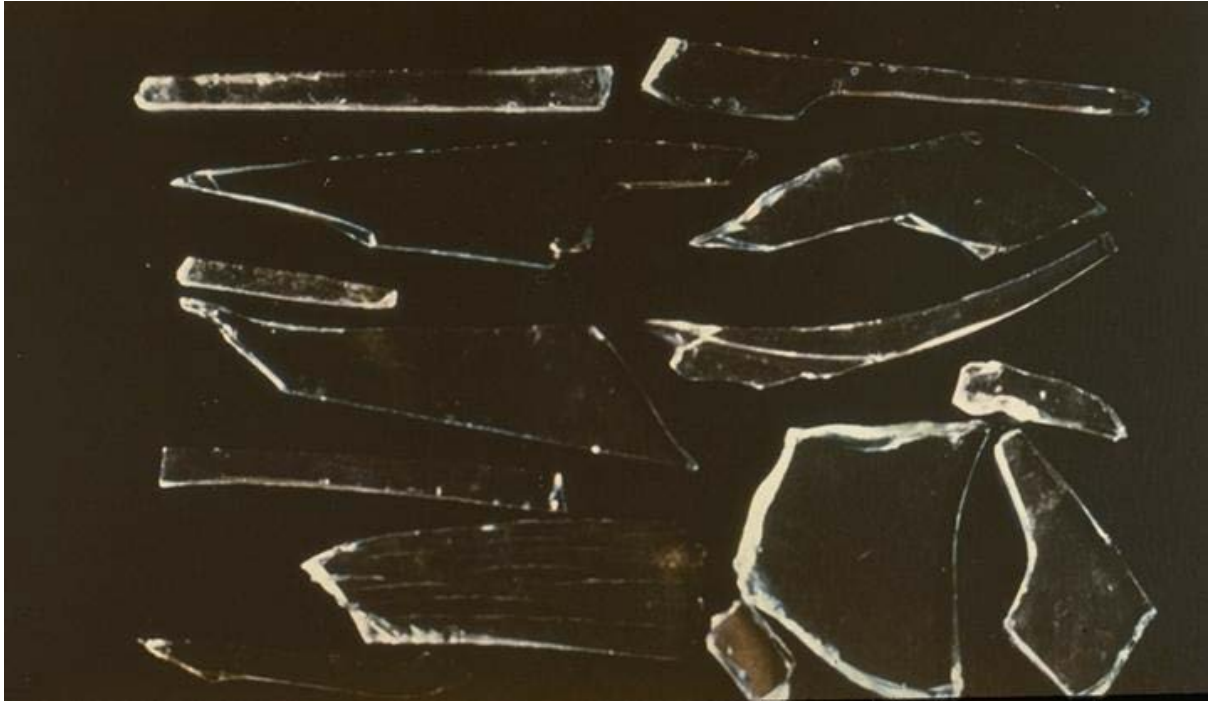
Figure 4-3. Window glass shattered by an explosion
