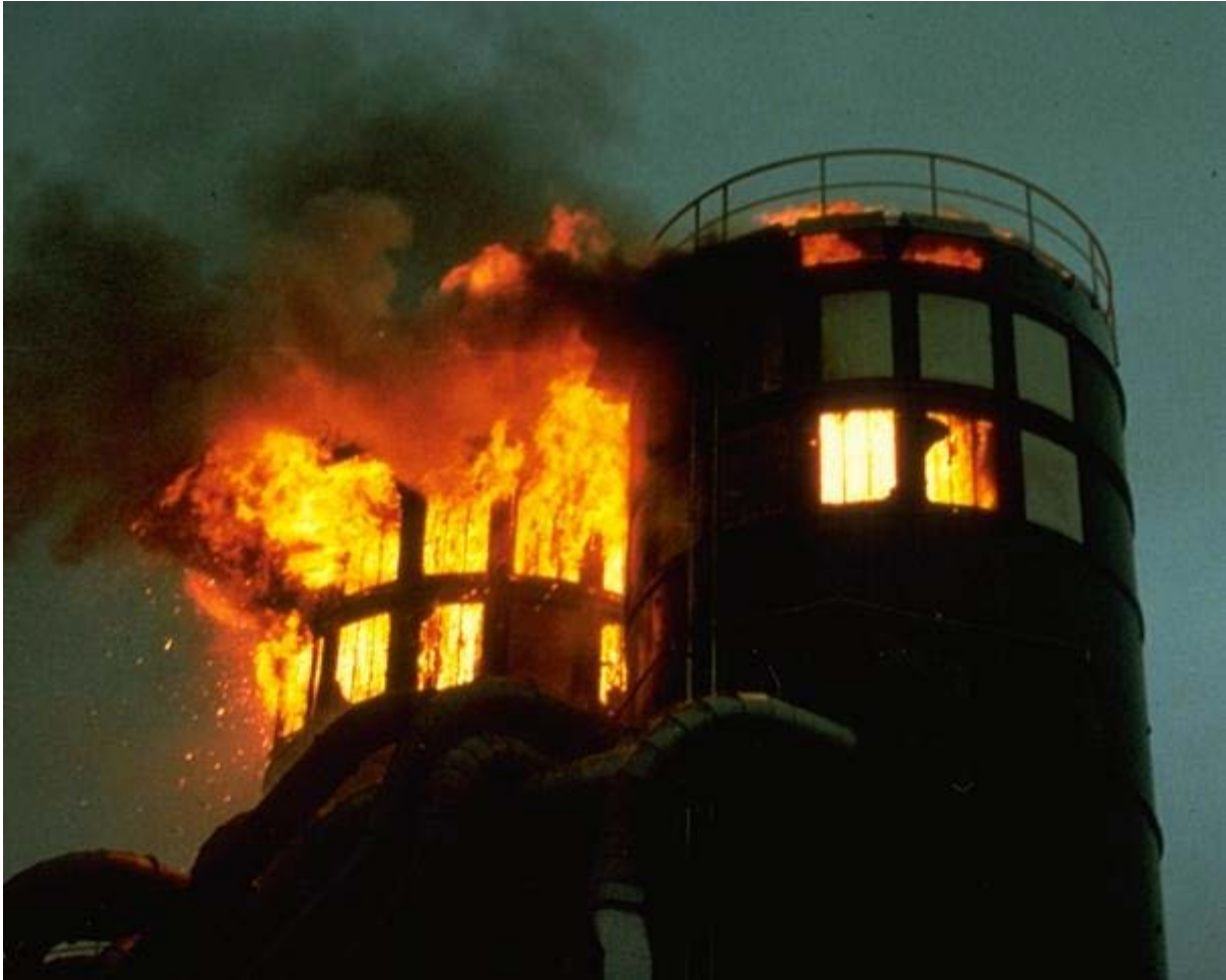
Figure 3-3. Subsequent fires after a dust explosion in a vented silo
