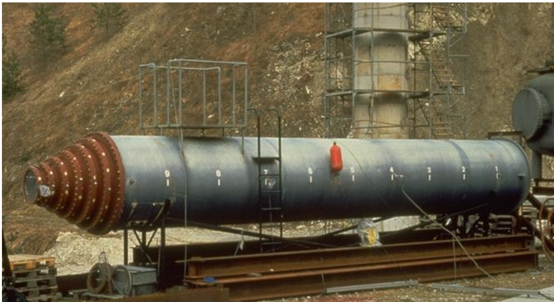
Figure 6-9. Elongated 20-m 3 -vessel with a L/D_e = 6.25
