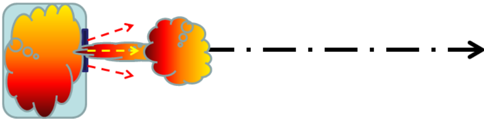
Figure 8-9. Explanation of the secondary explosion outside the vented vessel
