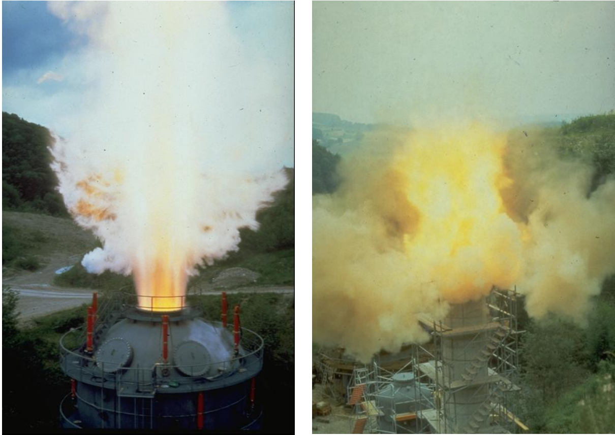
Figure 6-5. Explosion of standard dust dispersion in a vented 250-m 3 -vessel (left) and 20-m 3 -silo (right)
