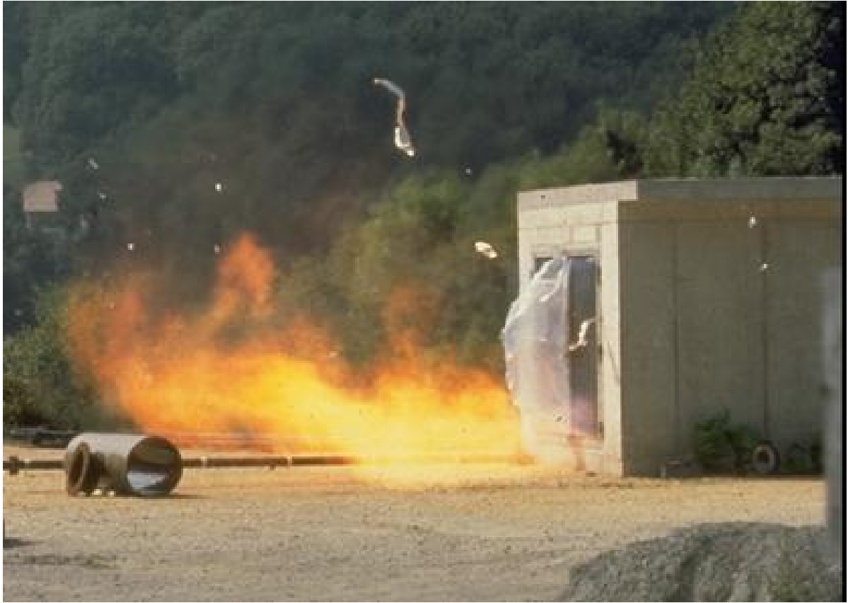
Figure 8-2. Gas explosion in a vented 25-m 3 -vessel with propane-air-mixture ignited at zero turbulence
