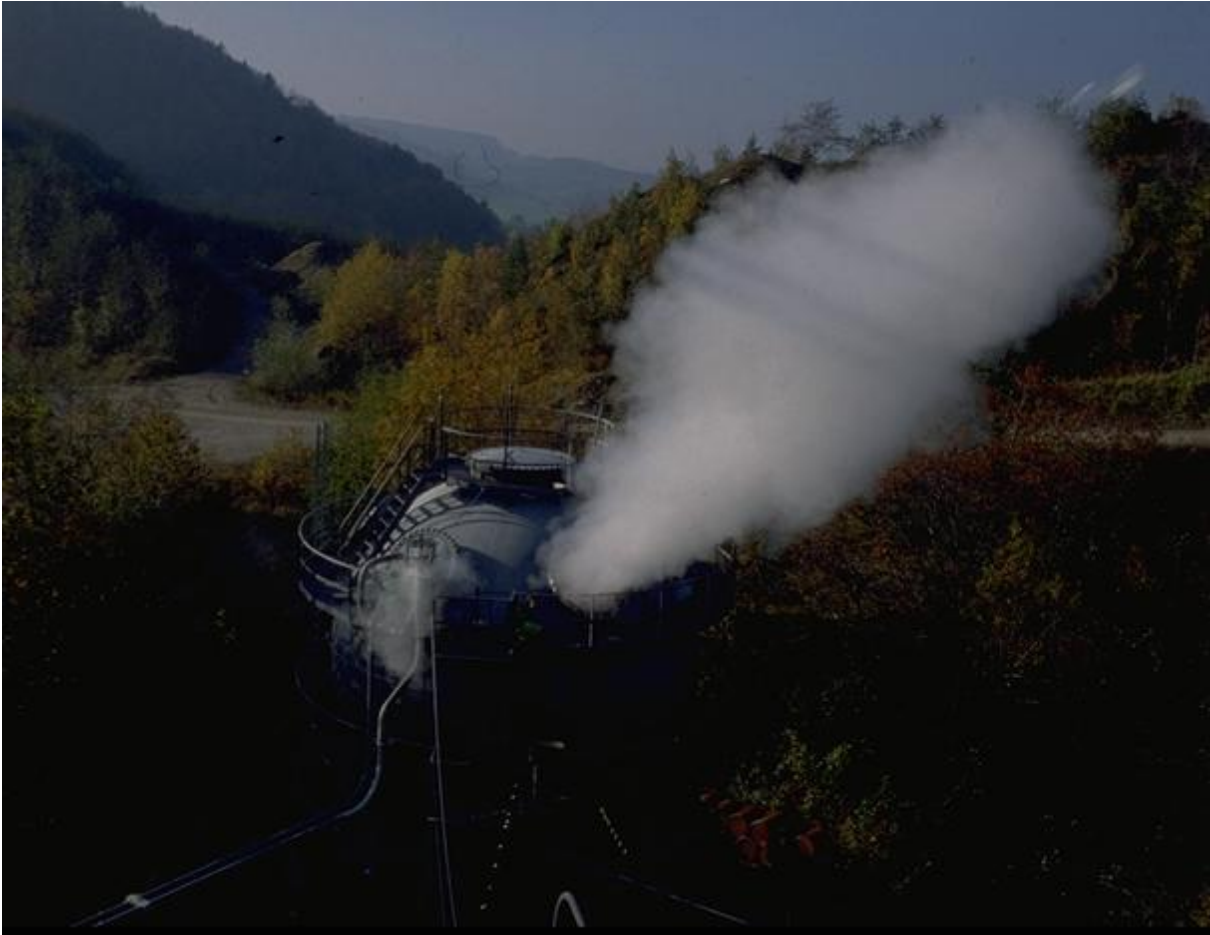
Figure 6-6. Explosion of a vented 250-m 3 -vessel introducing combustible dust through pneumatic transport in the form of pneumatic conveying
