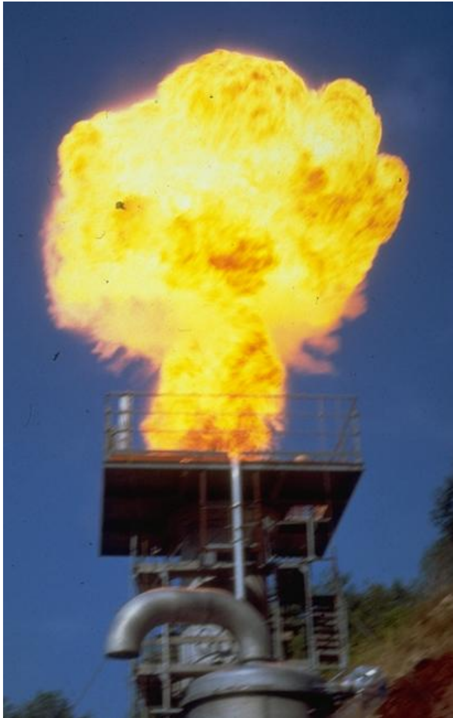
Figure 6-7. Explosion of a vented 20-m 3 -silo introducing combustible dust through pneumatic transport in the form of pneumatic conveying
