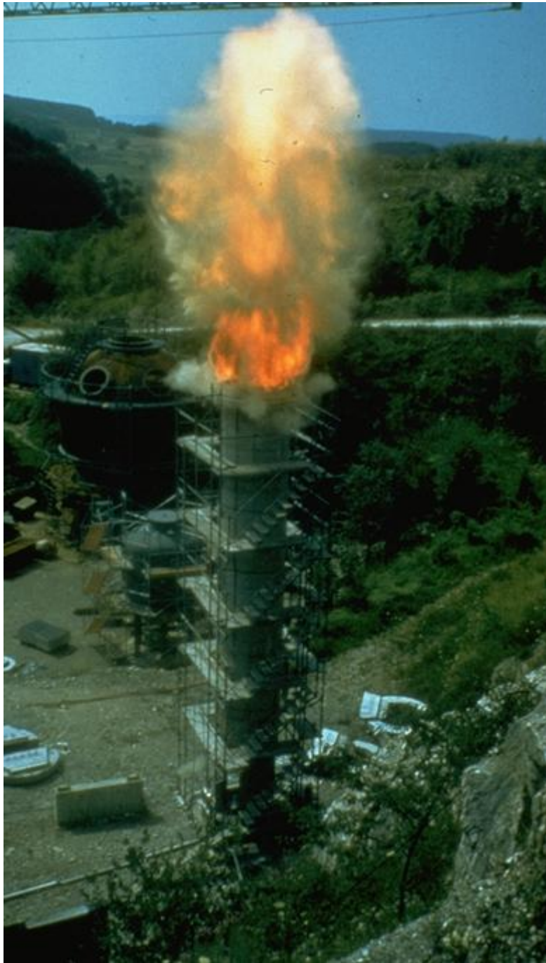
Figure 6-10. Vertical elongated 20-m 3 -silo ( H/D_e = 6.25 ) with explosion venting: dust explosion test
