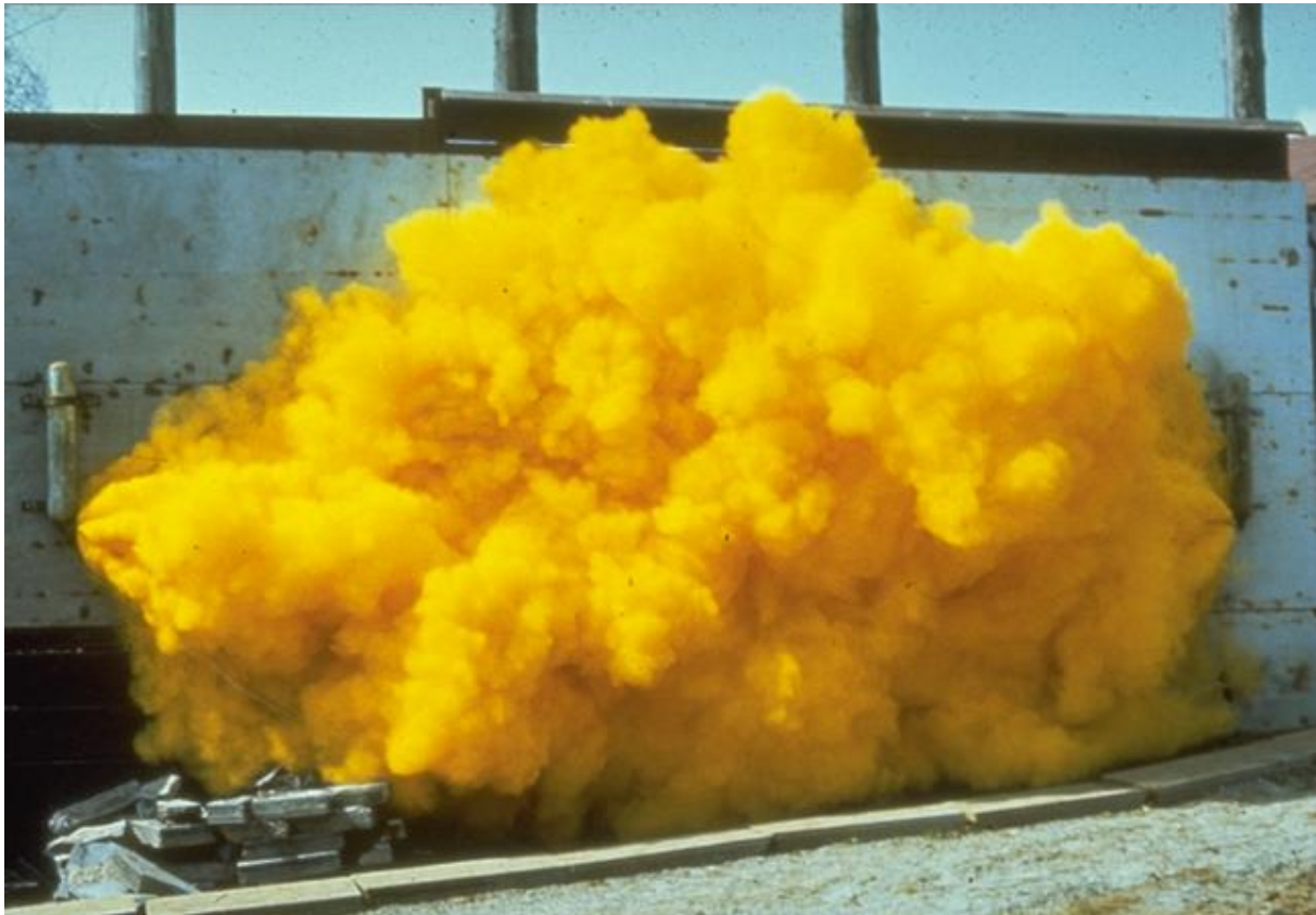
Figure 6-4. Standard dust dispersion by rapid release of combustible dust from storage containers
