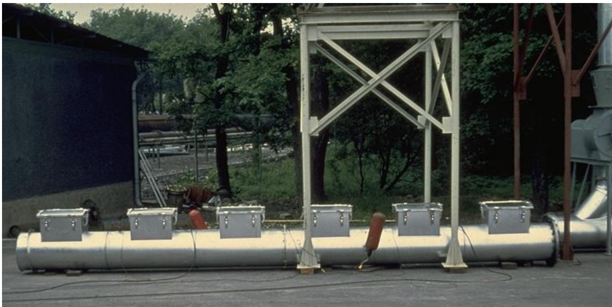
Figure 13-1. Pipeline shown with vent openings (vent openings closed with rupture disks) /5/
