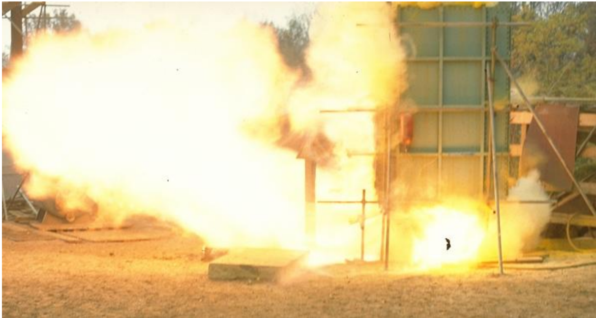
Figure 8-1. Dust explosion in a vented 7.5-m 3 -filter with standard dust dispersion
