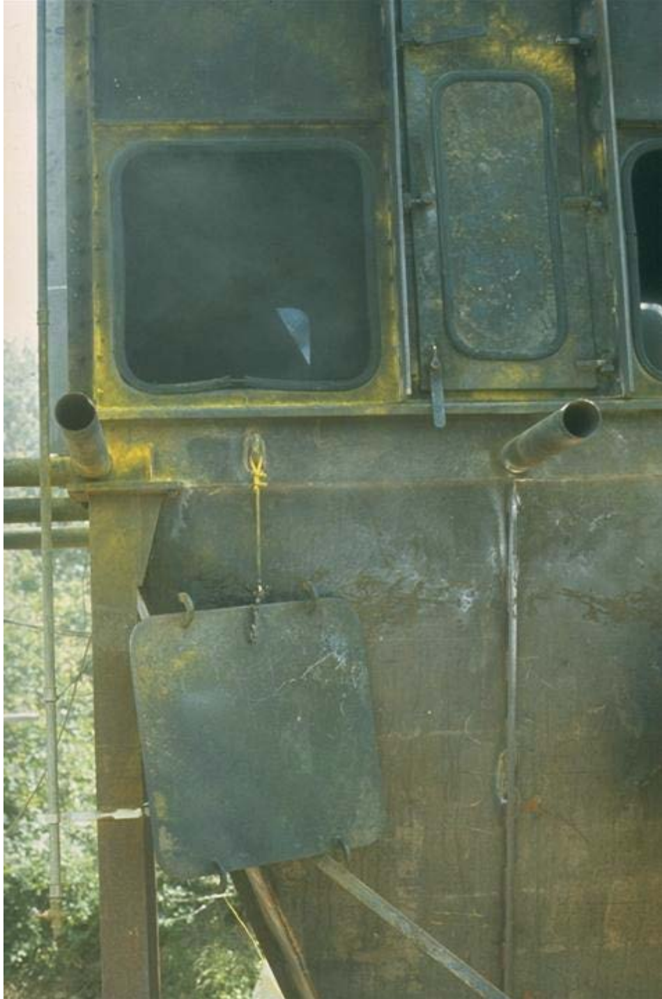
Figure 5-10. Explosion panels secured by 8 mm steel cables after explosion in filter housing
