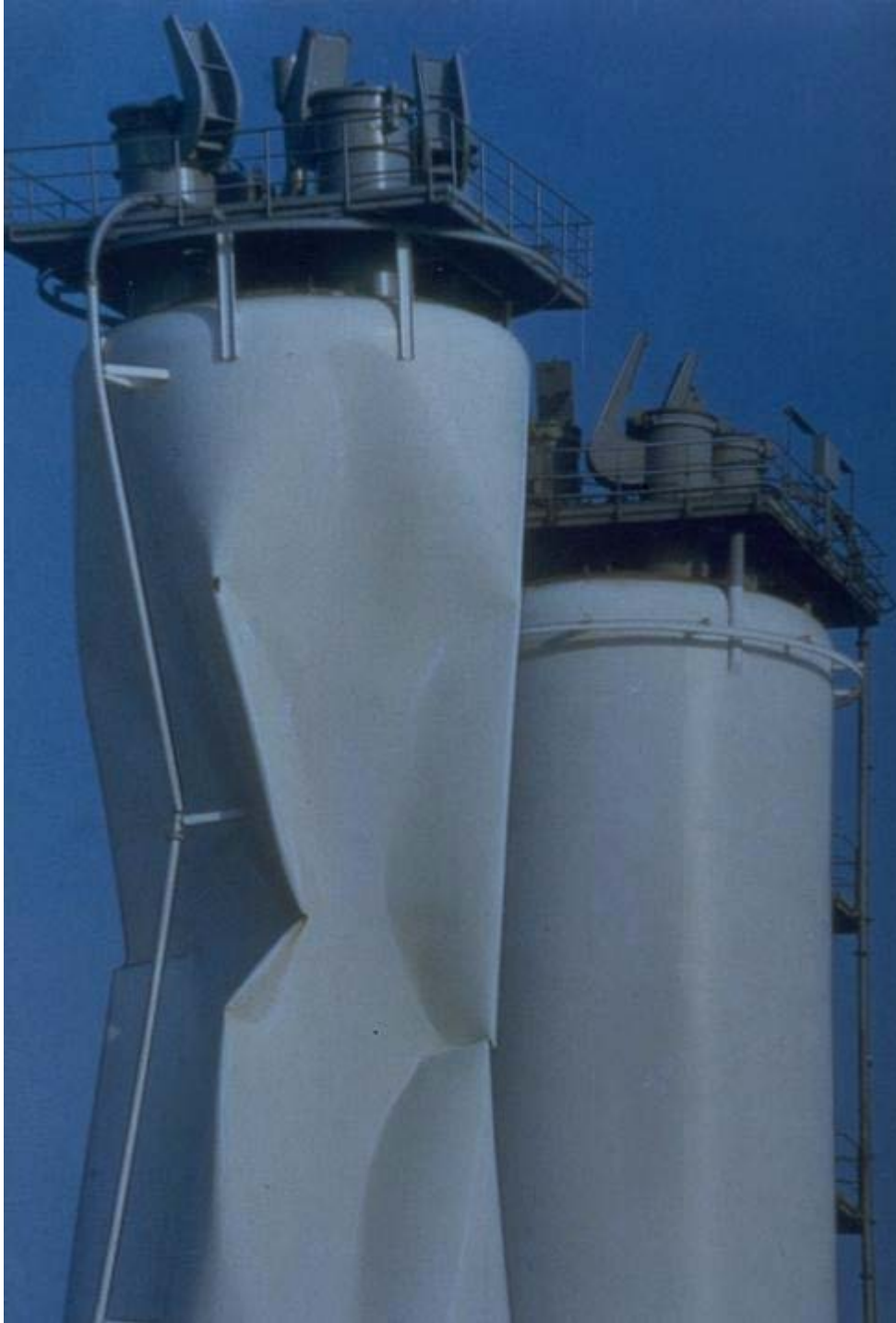
Figure 5-20. Silo, which was protected with explosion doors, destroyed due to vacuum /15/
