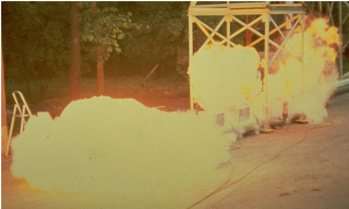
Figure 13-2. Wood dust explosion in a vented pipeline /5/
